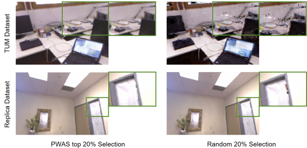
Figure 6. Visual reconstruction comparison under identical 20% transmission budget. PWAS Top-20% selection maintains structural integrity and detail preservation in challenging regions (green boxes), while random 20% selection results in noticeable structural loss and texture distortion.
