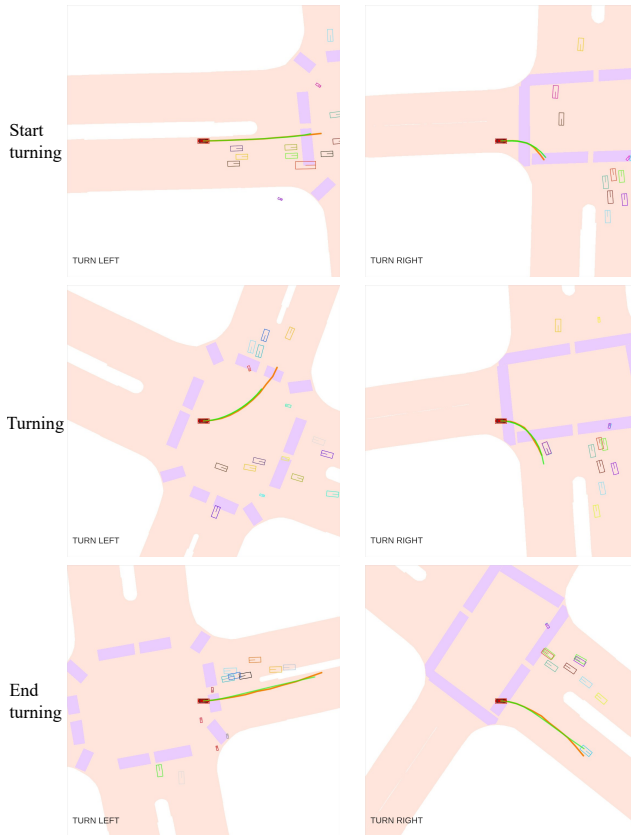
Figure 6. Qualitative comparison between the model trajectory (orange) and the ground-truth trajectory (green) in a complex turning scenario.
