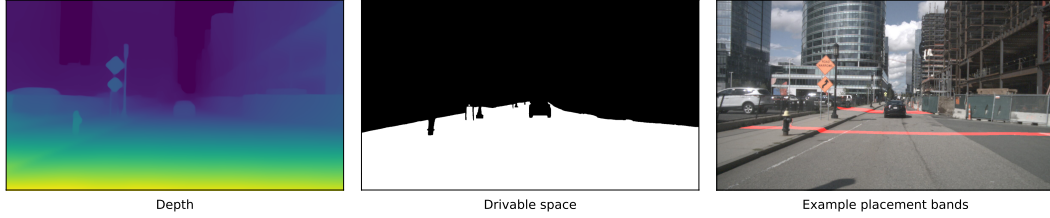
(b) Example frame with depth map and drivable space. We first draw a depth value and then select an area from the drivable space that is within a threshold \tau_d = 5 around that value. This results in placement bands from which a location is selected at random.
