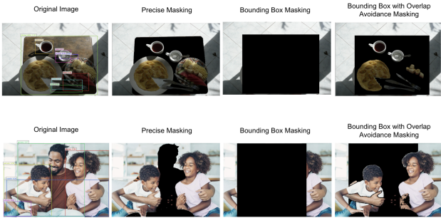
Figure 4. Comparison of masking strategies for object occlusion in PixelSHAP. (a) Precise masking follows exact segmentation boundaries. (b) Bounding Box Occlusion with Adjustment (BBOA) uses expanded boxes to ensure complete occlusion while minimizing interference with neighboring objects. BBOA consistently achieves better attribution performance across different scenarios.
